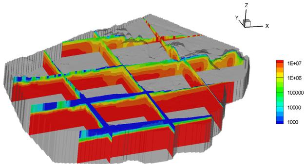
Figure 9. Mean lifetime expectancy for density dependent flow (Years)
