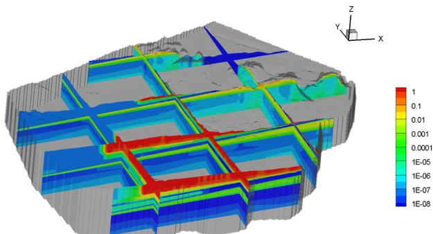
Figure 5. Steady-state flow velocities (M/Year)
